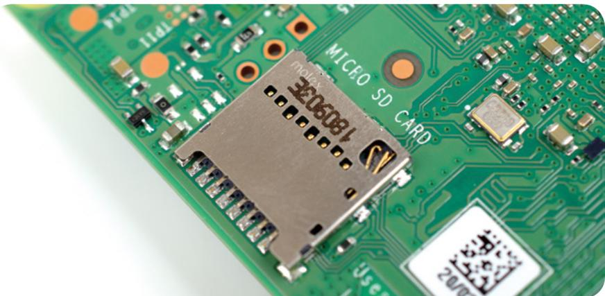
▲ **Figure 1-15:** Raspberry Pi's microSD card connector
