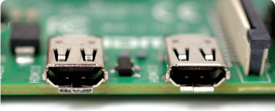
▲ **Figure 1-10:** Raspberry Pi's micro-HDMI ports
